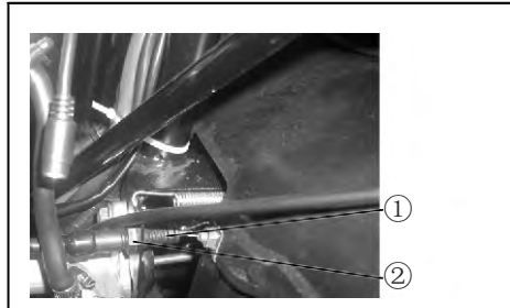
1. Brake light switch 2. Adjusting nut
