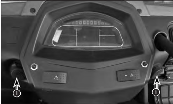
1. 12V DC outlets
