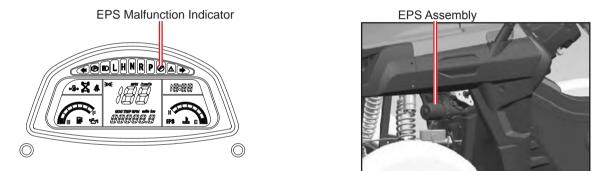
Each trouble code consists of 2 digits, denoted by the times of long flash and short flash of EPS MIL indicator. If there is a failure, the EPS indicator will start to flash. Do NOT switch off the machine. Check the flash sequence of EPS indicator. Write down the flash sequence and contact your dealer for diagnosis.
