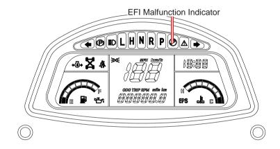
If there are multiple codes detected, the system will wait approximately 3 seconds and display the next code. Any codes displayed will disappear once the problem has been diagnosed and repaired by your dealer.
