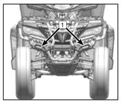
A full HDPE skid plate system is installed to protect the bottom of the ATV from rocks, sticks, and other objects.
