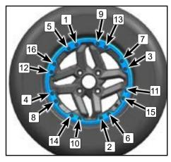
Check to ensure the tire is in the center of wheel. Reposition it as necessary.
