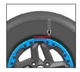
Beadlock ring bolts (Final torque): 106 in-lb (12N·m ± 1N·m)
