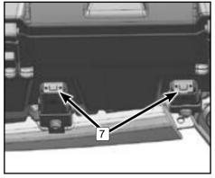
Press the lock button 7 to release the lock. Pull out the lock hook 6 to open the lock.
