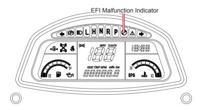
If there are multiple codes detected, the system will wait approximately 3 seconds and display the next code. Any codes displayed will disappear once the problem has been diagnosed and repaired by your dealer.
