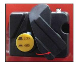
On-Command 2WD / 4WD / 4WD-LOCK Switch Operation
